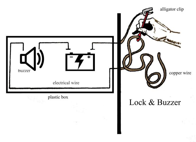
To represent IFGS lockpicking, a lock and a buzzer are connected to form an open, complete circuit (see diagram), which will only close if a character touches his lock pick to the bare copper wire of the lock. The buzzer apparatus is usually contained in a portable box that can be moved from encounter to encounter (often by the GM). Constructing a Lock The following items are required for lock construction, and can be obtained at most hardware stores:
