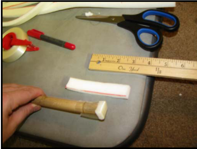
Figure 13: Attach a square of foam to the core's tip
