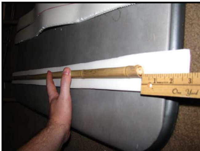
Figure 9: Mark 2.5" to leave as padding for the blade's tip
