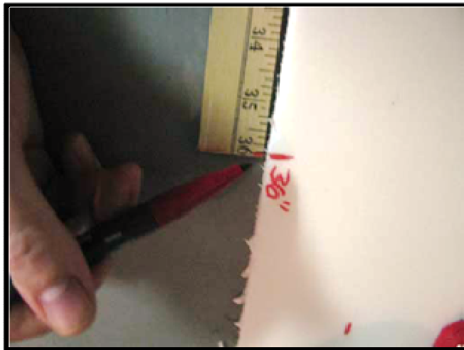
Figure 4: Mark the long edge of the foam at 36"
