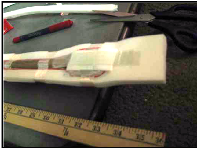
Figure 19: Attach 1/8" foam to cover the thrusting tip
