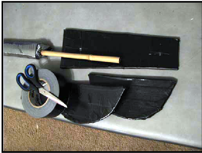
Figure 39: Cover the guard pieces with duct tape
