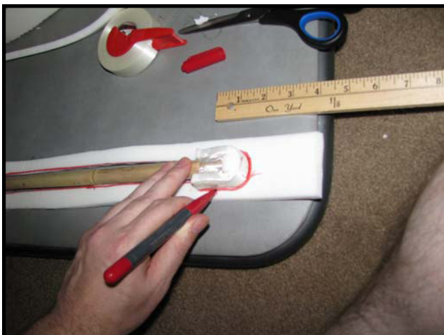
Figure 15: Trace around the padded tip
