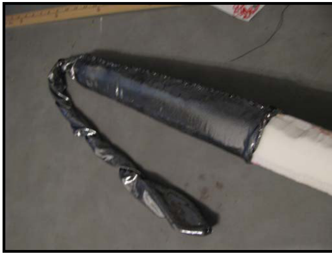
Figure 31: Carefully stretch the sock over the blade
