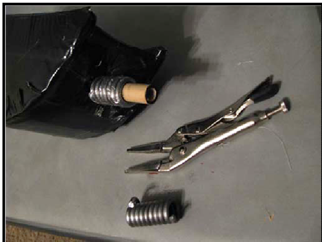
Figure 41: Wrap the core with lead tape to adjust balance
