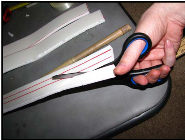
Figure 11: Cut out the marked center portion
