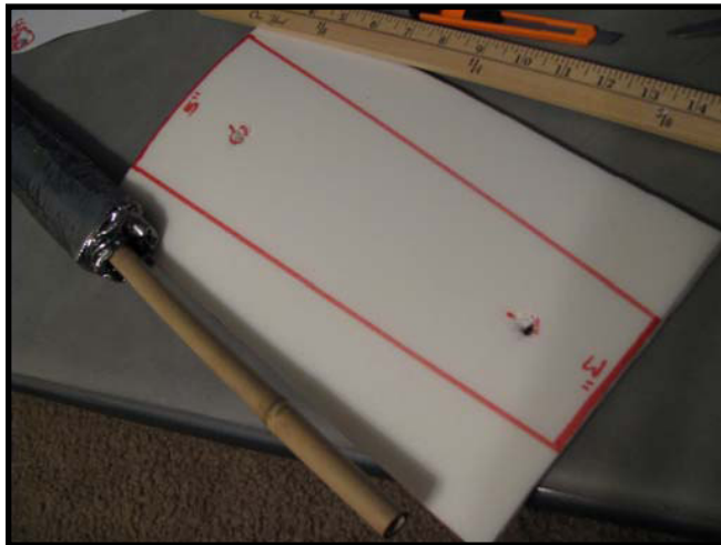
Figure 35: Cut small holes for the core
