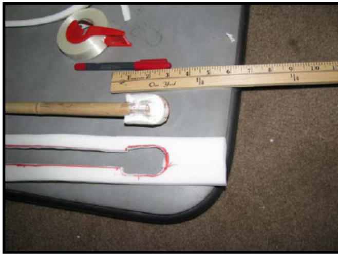
Figure 16: Trim the blade piece to match the padded tip
