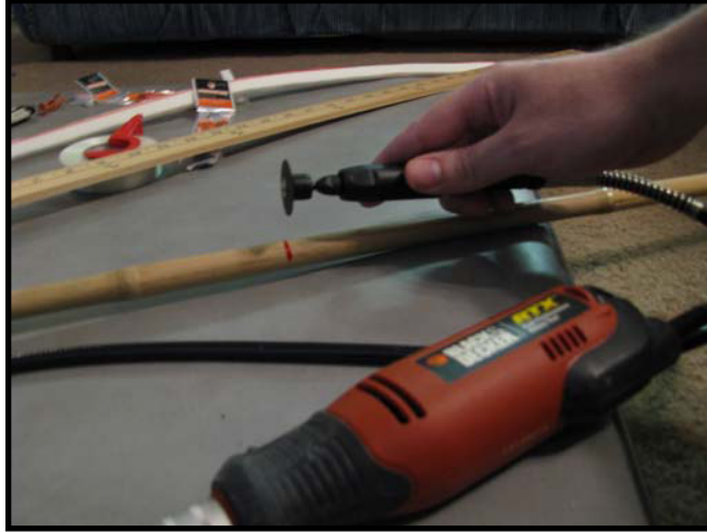
Figure 8: Cut the core to a length of 44"
