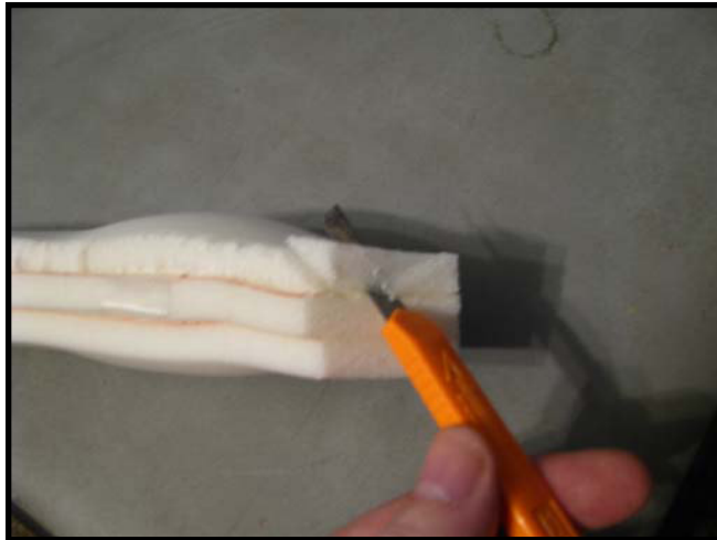
Figure 26: Cut a beveled edge into the outside layers of the tip
