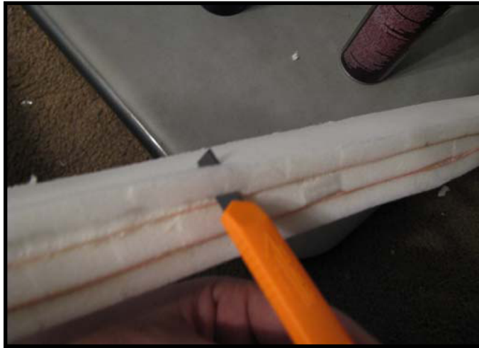
Figure 28: Cut a beveled edge into the outside layers of the blade
